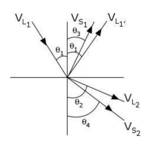
VL1 is the longitudinal wave velocity in material 1.
