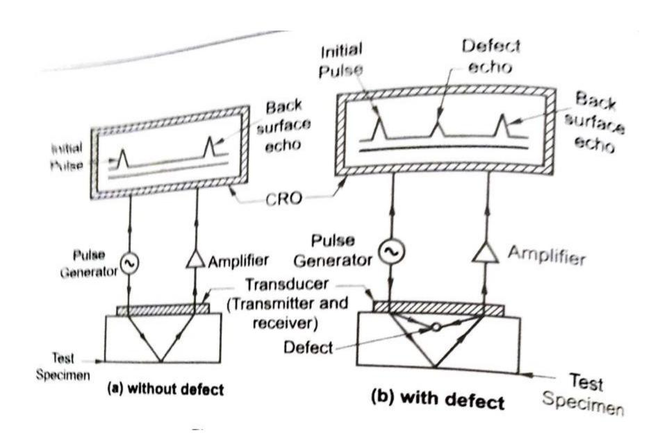
The pulse-echo technique allows testing when access to only one side of the material is possible, and it allows the location of reflectors to be precisely determined.
