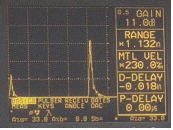
Digital display showing loss of received signal d ue to presence of a discontinuity in the sound fiel d.
