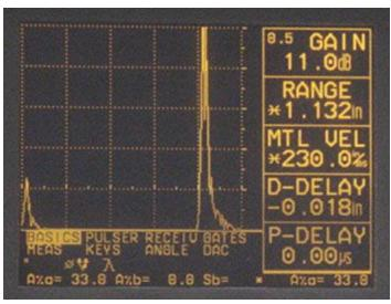
Digital display showing r eceived sound through ma terial thickness.
