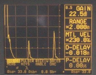
Digital display showing t he presence of a reflector midway through material , with lower amplitude ba ck surface reflector.
