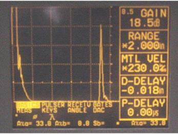
Digital display showin g signal generated fro m sound reflecting off back surface.
